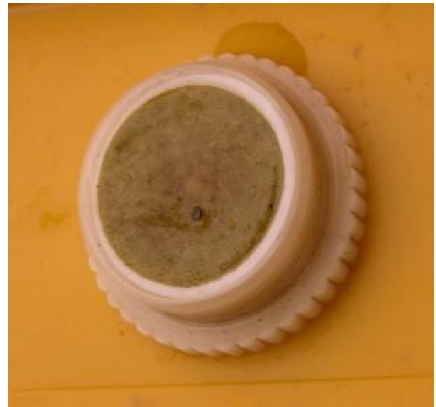
Figs. 42 To index chlorophyll and phaeopigments, we filled a syringe with pond water, attached to the hole at the top of the filter illustrated at left. After passing a known amount of pond water through the filter, we opened the filter (see image on right) and removed the filter paper for subsequent analysis. This filter came from a pond with high amounts of dissolved algae; if there had have been no algae, the paper would have been white.
