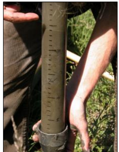
Fig. 10. An example of a pond core. The clear plastic tube was held within a metal tube that was lowered into the sediment. It was then capped, returned to the surface, and removed from the metal case.
